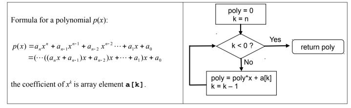
Use the <u>second</u> formula for p(x) in your Java code, as shown in the flowchart at right. This formula is faster and usually more accurate. It is faster because you don't need to compute powers if x. The flowchart can be implemented as an indexed **for** loop.
